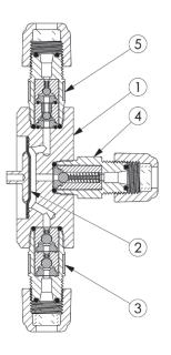
The AUTOPRIME<sup>™</sup> liquid end consists of 5 functional elements. They are the Head (1), Diaphragm (2), Suction Check Valve (3), Discharge Check Valve (4) and Autoprime Valve (5).
